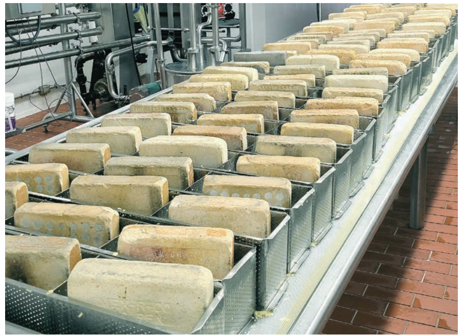
Widmer's Cheese still makes Brick cheese much the same way as it has for the past 100 years, pressing the Brick loaves with the same well-worn five-pound bricks that his grandfather, John Widmer, used to press the cheese after it has been placed in the forms.
